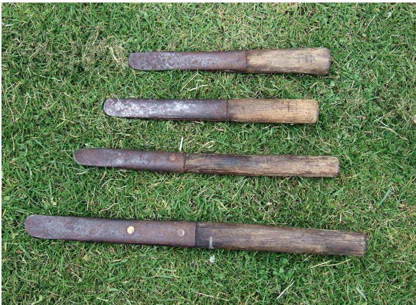
Fig 7 Rippers used for rinding. The top ripper is approximately 30 cms (12 ins) long. (Rippers courtesy of Tony Gunn. Photograph: Nigel Baker.)
