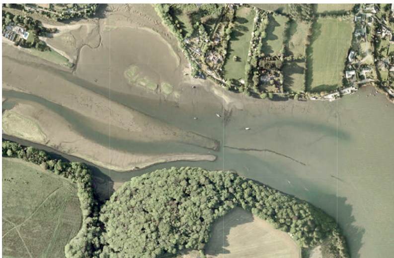
Fig 1 Various lines of faggots are still visible in the Carnon Creek....they were used for constructing “training banks” that directed the river flow to better scour the navigable channel (Nicholas Johnson, pers comm, 2024). (Photograph: Nicholas Johnson.)
