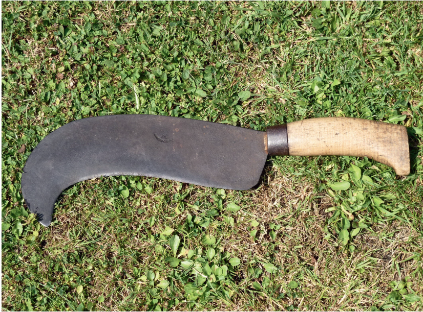
Fig 6 A 'patch hook' belonging to the author; 40 cms long (15.75ins), the maker's mark is illegible. It is very light, made of the finest steel and very rarely requires sharpening. (Photograph: Nigel Baker.)
