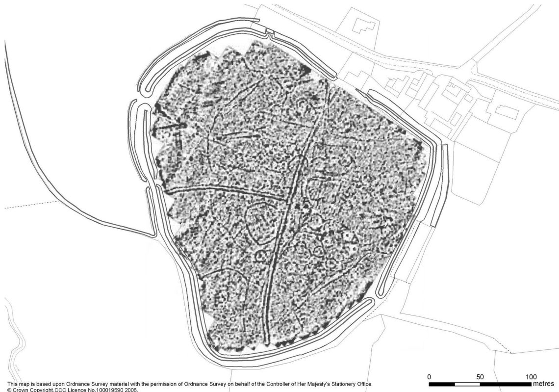
Fig 5 Greyscale results of a fluxgate radiometer survey (GSB Prospection) of the interior of Gear, with current Ordnance Survey mapping.
