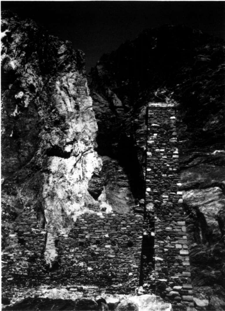
Fig 5 Bradda Head, Isle of Man. Opencut workings on a copper vein exposed in the cliff face. Photograph by courtesy of Dr David Jenkins
