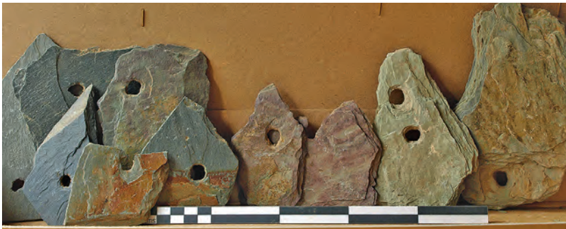
Fig 25 Context (107), small slate fragments that show consistent peg hole size and considerable geological variety. (Photograph: Eric Berry.)
